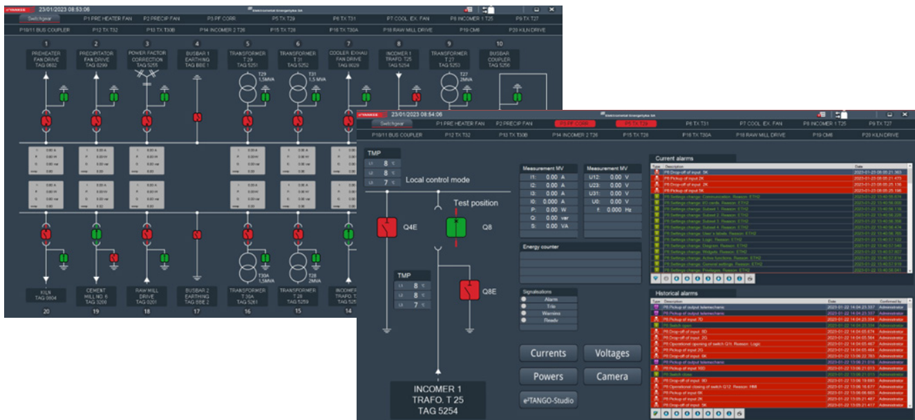
Synoptic diagram of the e 2 YANKEE system for switchgear in the MV substation
