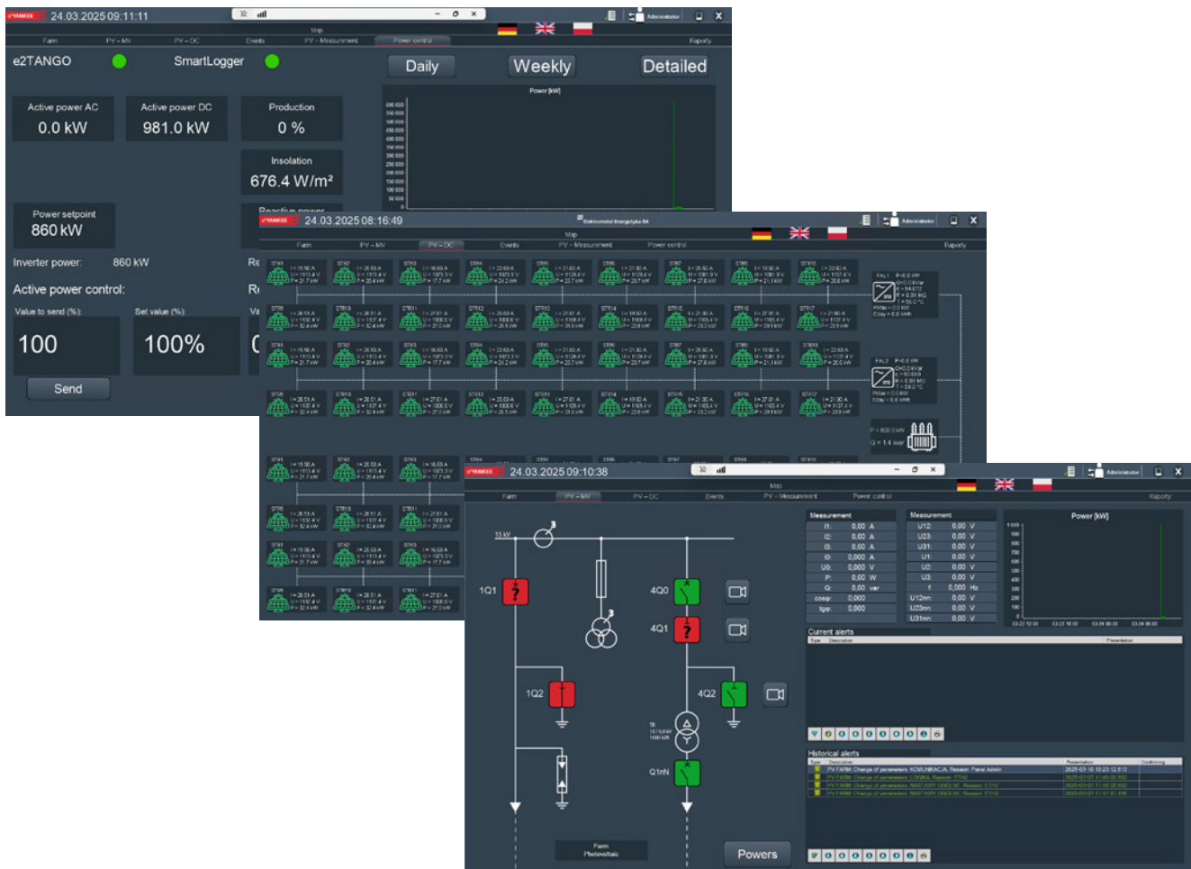
Synoptic diagram of the e 2 YANKEE system for photovoltaic farm and MV substation
